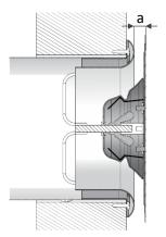
a= adjustable distance between the glass plate and the body of the valve with the option of regulating air flow-through rate
